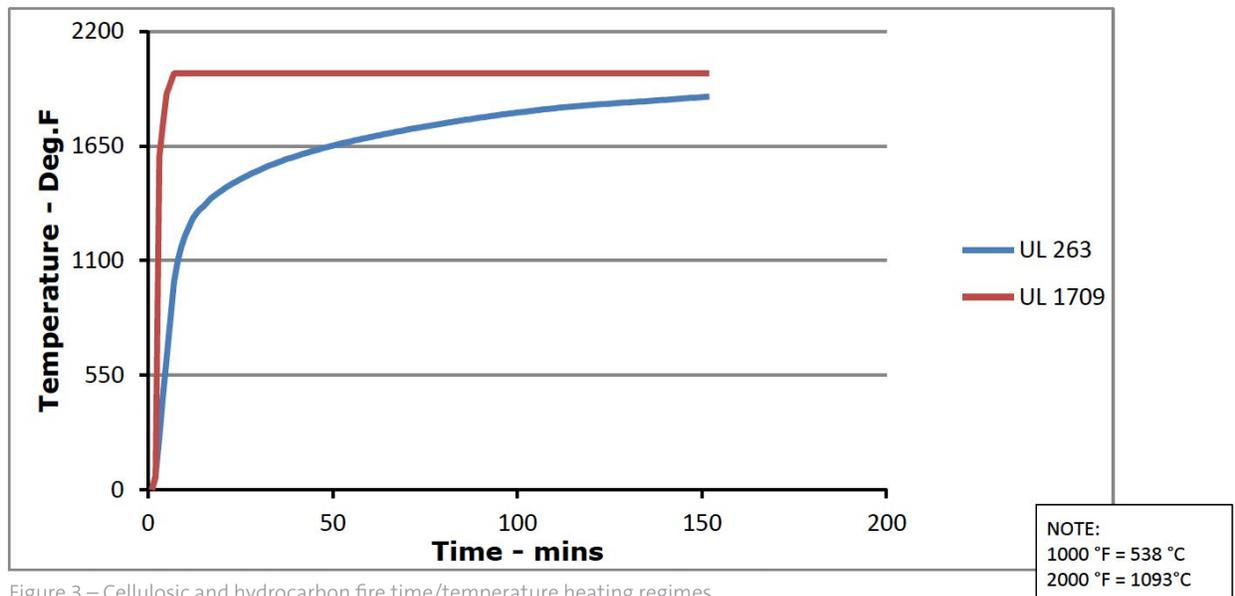
Figure 3 – Cellulosic and hydrocarbon fire time/temperature heating regimes
