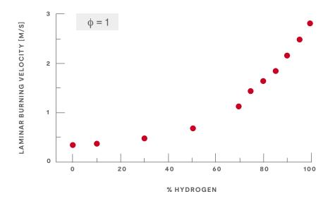
Figure 4: Flame speed of hydrogen-natural gas blend with various percentages of hydrogen at  $\phi = 1$ .  $\phi$  is the equivalence ratio, so this is assuming a stoichiometric (complete combustion) air-fuel ratio; this infers these burning velocities may be different for lean burning conditions.<sup>30,31</sup>
