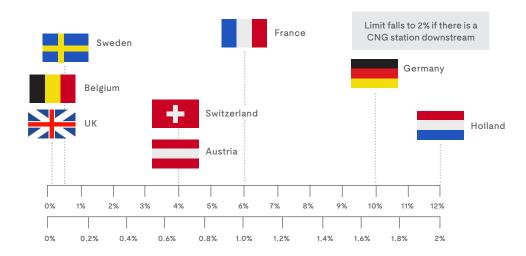
Figure 5: Hydrogen limits for natural gas pipelines in several European countries. <sup>19</sup>
