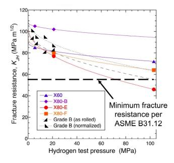
Figure 1: Fracture resistance of X60 and X80 steels with increased hydrogen (100%) test pressure.<sup>20</sup>
