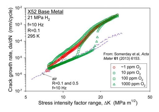
Figure 3: Data from testing with X52 steel illustrating that the presence of 1000 ppm (1%)  $O_2$  in hydrogen gas can reduce the crack growth rate back to that experienced in air. For X52 steel, this is true for a stress intensity factor ( $\Delta K$ ) range up to around 18 MPa m1/2.<sup>14</sup>
