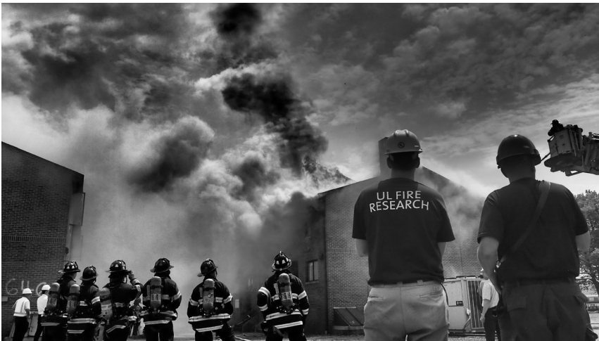
In an unprecedented series of controlled burn experiments at abandoned buildings on Governors Island in 2012, UL partnered with the New York City Fire Department and the National Institute of Standards and Technology to test how fires spread in homes and to determine the most effective and efficient way to suppress the fire and save potential occupants.
