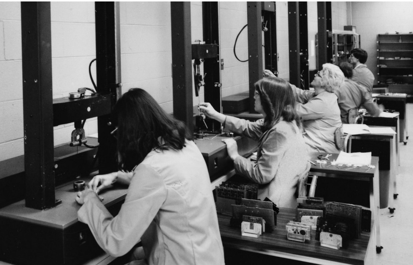
Technicians at UL's Northbrook laboratory conduct tension and compression tests on appliance wiring material (1983).
