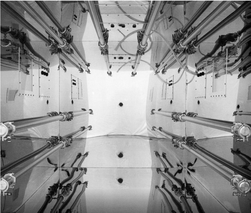
The UL Environmental Testing Chamber located in Atlanta, Georgia, tests chemical emissions (2013).
