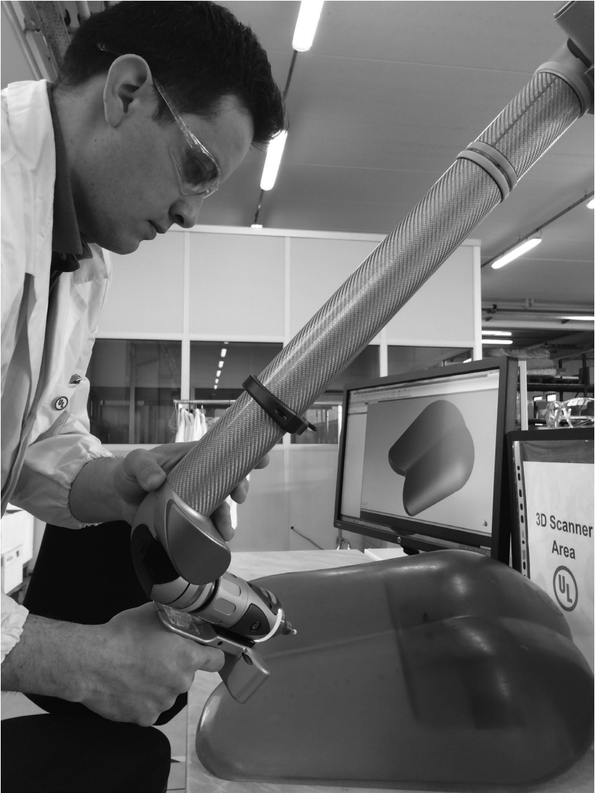
A technician from UL Italia Cabiante uses a portable coordinate measuring machine (CMM). This machine analyzes a product's quality by performing 3D inspections, tool certifications, CAD comparison, dimensional analysis, reverse engineering, and more (2016).
