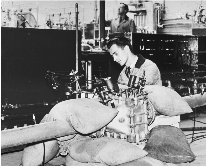
The War Department urgently needed UL's services during WWII, to develop safety standards during the rapid expansion of factories and new manufacturing processes. Here a technician sets up an explosion test for a flame arrester.
