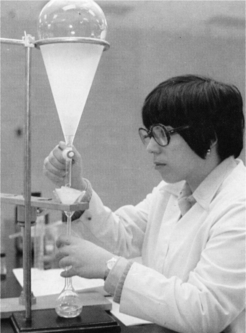
A UL technician measures oily water samples to determine compliance with U.S. Coast Guard regulations for water pollution (1979).
