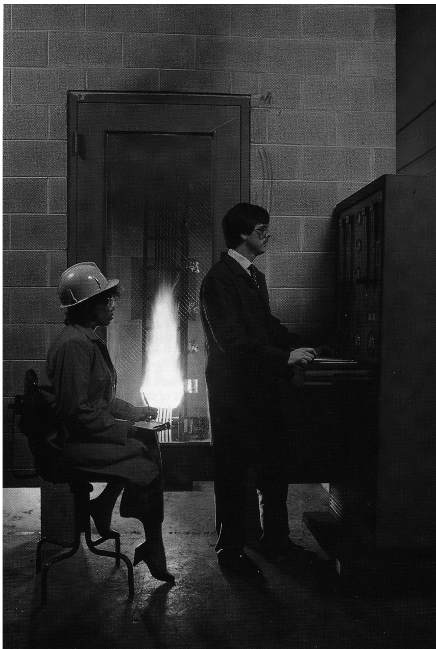
UL conducts fire tests on cable to help protect vital communications and electrical services (1989).
