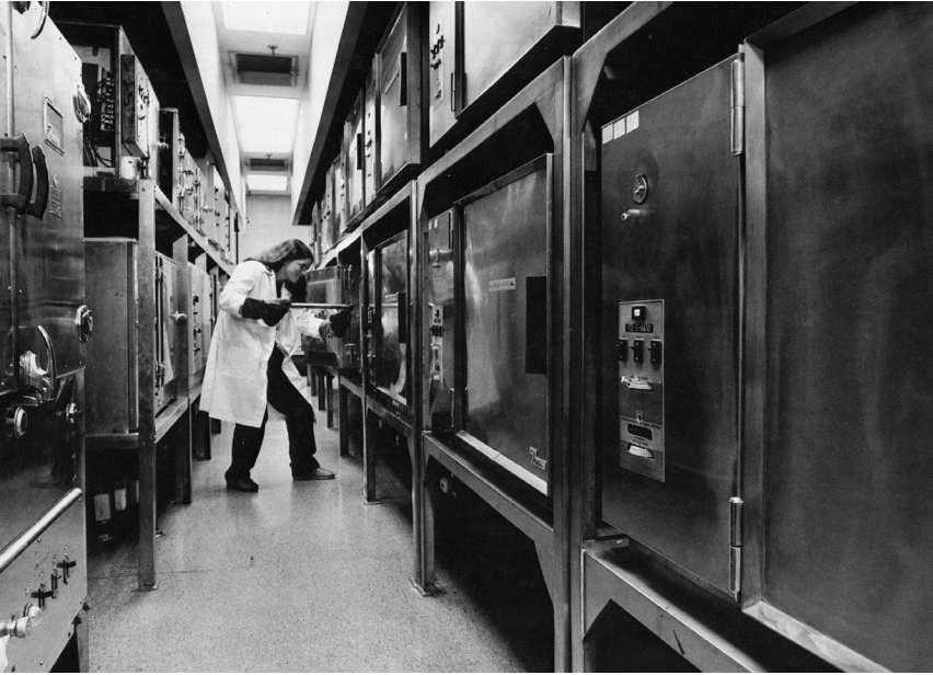
A UL employee places rubber and plastic materials into ovens to accelerate aging and conditioning (1980).
