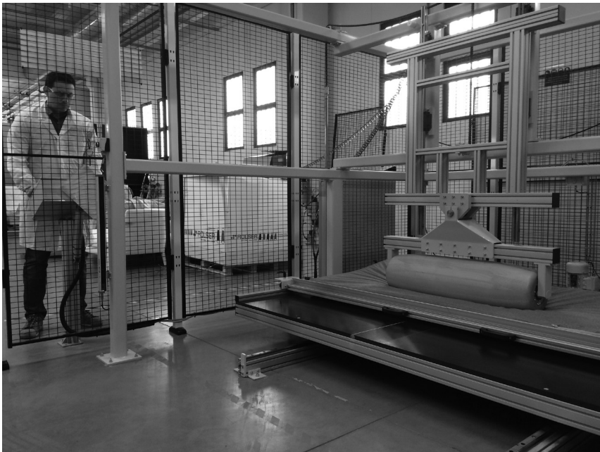
Mattresses are one of the most utilized items in a home, enduring six to nine continuous hours of use per day. With this equipment, UL can determine the safety and comfort of mattresses and bedding (2016).
