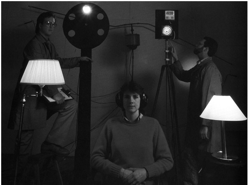
In 1990, UL conducted light perception tests on hearing-impaired individuals to determine the light signal intensity necessary for manufacturers to design an effective fire-alarm signaling device.
