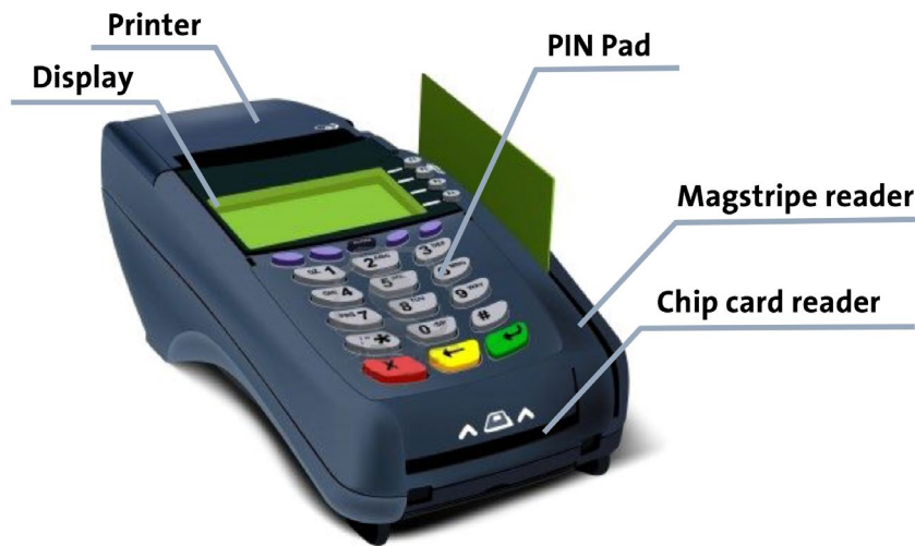
Figure 3. Typical POS terminal hardware components
