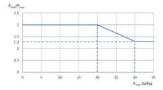
Figure 01: Ratio between test pressure and maximum working pressure
