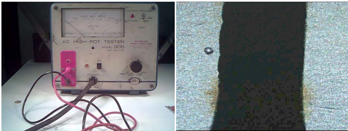
Figures 2ab - High-Voltage Source Used in Withstand Voltage Test; Test Pattern after Electric Arc
