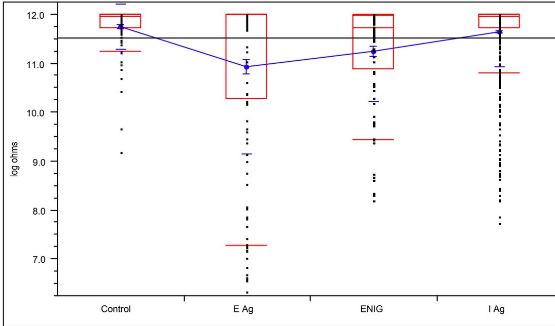
**Figure 7 - Electrochemical Migration Test Results at 596 Hours**
