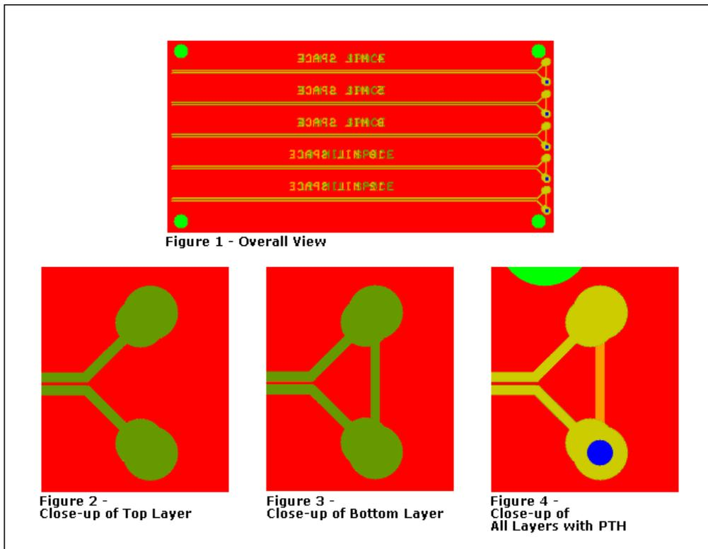
**Figure 4 - Test Board Design Recommendations for Use in Submissions to a UL-Certified Lab**
