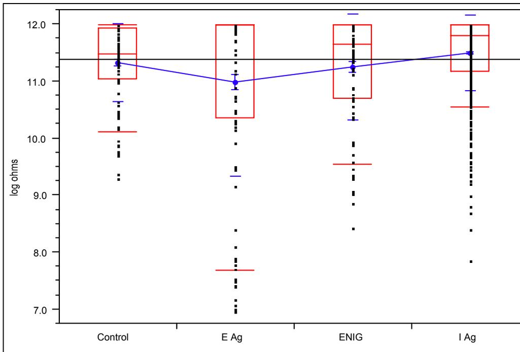
**Figure 6 - SIR Test Results at 96 Hours**
