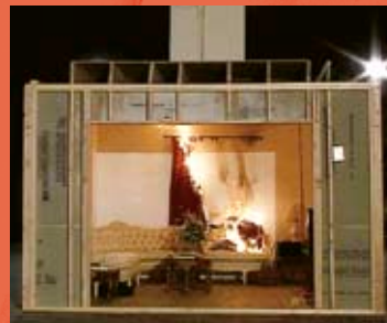
Left: Legacy room Right: Legacy Room at 5:00 after ignition
